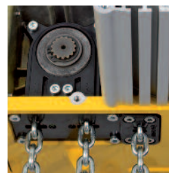
Integrated limit switches, and easily removable chain sprocket & guide.
