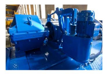
**Each winch** consists of a main gearbox, featuring either two or three reduction stages, connected to a three-phase asynchronous motor of short-circuited type.
